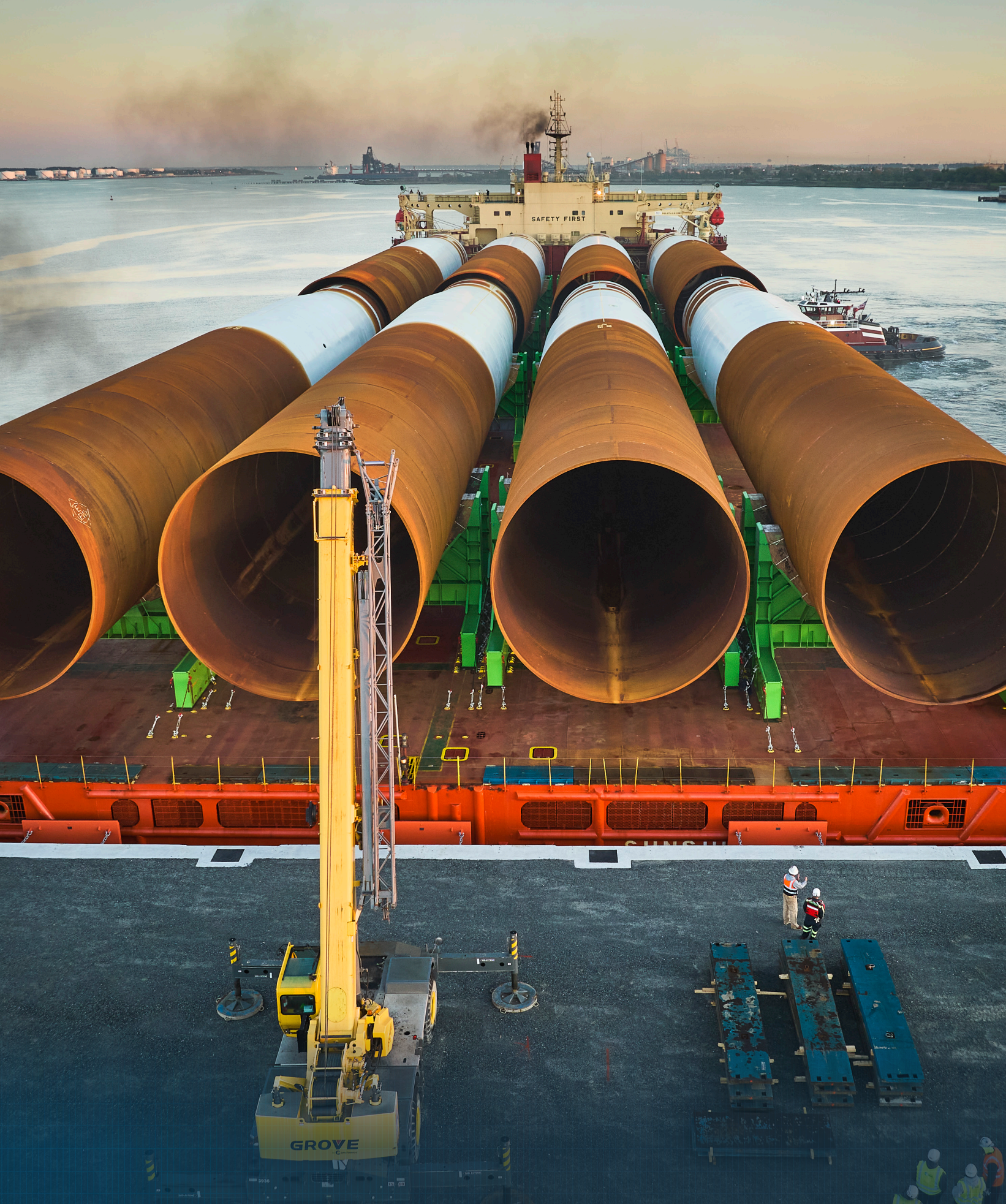
Coastal Virginia Offshore Wind monopiles ready to be discharged at Portsmouth Marine Terminal.
